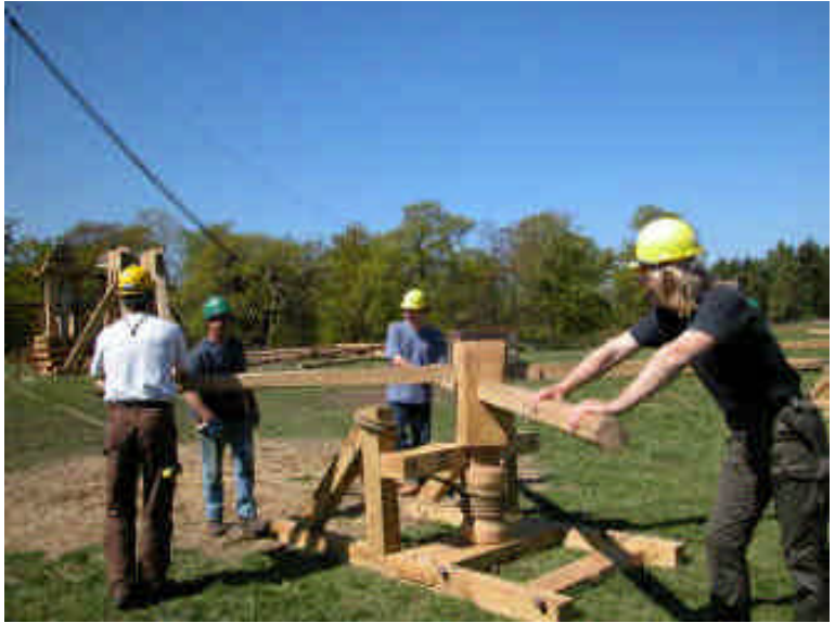
Twin A Frame lift to position 8.5 tonne catapult body on its stand
